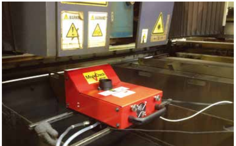
ModeCheck with optional MLA, profiling a CO 2 cutting laser with its processing head installed
